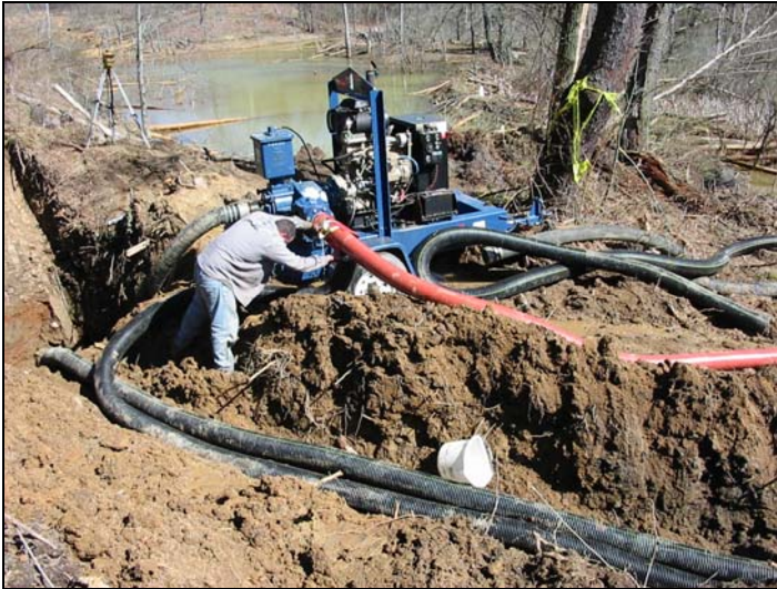
Pumping Test Pit 1 to monitor mine pool response at piezometers, "blowout" (future EWS), and Test Pit 3 (future Secondary Drain). (April 9, 2005)
